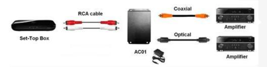
b. Digital input convert to Analog output:
