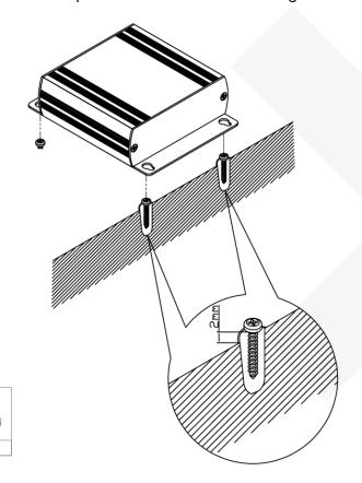
Step 2: Place AD001HD4-4K on the platform and fit its holes in the corresponding screw positions.
