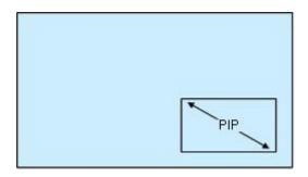
Button as PIP sub-screen dimension setting, press ◀ to decrease PIP sub-screen dimension, press ▶ button to enlarge PIP sub-screen dimension.
