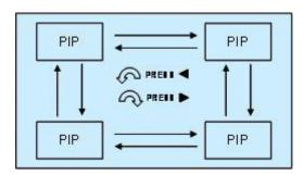
Button as PIP sub-screen display position, press ■ Counter-Clockwise to switch, press ► Clockwise switch When press ■ two buttons together, two inputs can be switched between the main picture and sub picture.
