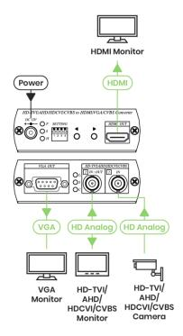
\* Enable HDMI, VGA, CVBS outputs: display 3 videos simultaneously.
