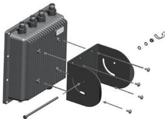
**Step 2:** Lock the 2 stainless tight hoop strips around the pole by passing through the mounting bracket and lock the fastening screws.
