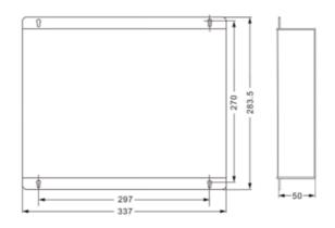
IP audio terminal NAS-8505B is suitable for wall-mounted installation , use 4 plastic expansion sleeves (F7) and 4 semi-round head tapping screws (M4 \* 25) provided with the equipment , refer to the installation dimensions below to fix the device on the wall.
