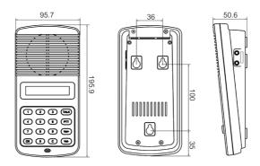
Installation instructions: The terminal can be installed on the desk or fixed on the wall by three cross screws.
