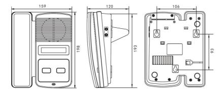
Installation instructions: The terminal can be installed on the desk or fixed on the wall by three cross screws.
