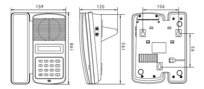
Installation instructions: The terminal can be installed on the desk or fixed on the wall by three cross screws.
