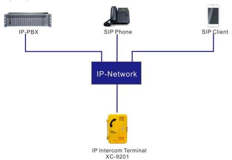
Application3: IP Intercom Terminal XC-9201 can be connected with external horn speaker( $8\Omega$ ), it can receive the broadcast tasks from server and the sound output from the horn speaker; Meanwhile, it supports one-button call with IP Paging Microphone.
