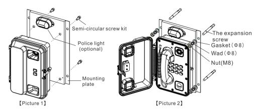
**Step 1:** secure the main unit to the mounting plate using the semi-circular screw kit in the accessory. As shown in Picture1. (If don't select alarming light, then the mounting plate and terminal is already secured, users can install it directly following step 2)
