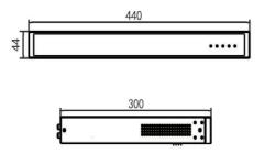
IP amplifier XC-9508 in rack-mounted installation with 4pcs of white washers head screws (M3\*5). Please refer to the following dimension diagram to put device in suitable cabinet
